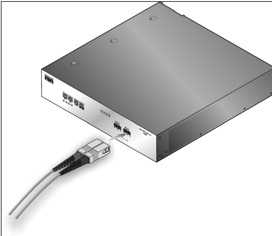
Figure 16: Cabling the GBE Interface
