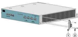
Figure 3: Attaching the Mounting Brackets (2-post)
