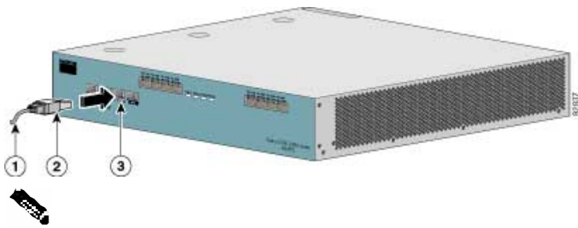
Figure 13: Cabling the Management Port
