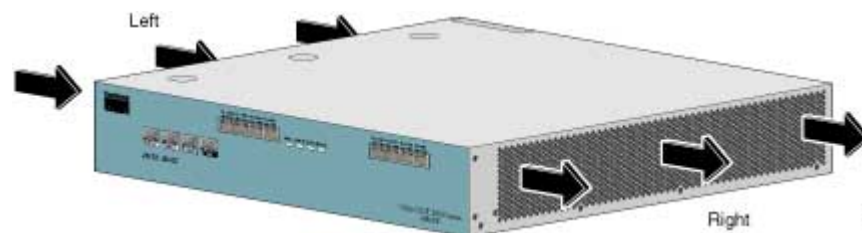
Figure 4-2: Airflow Through the SCE Platform
