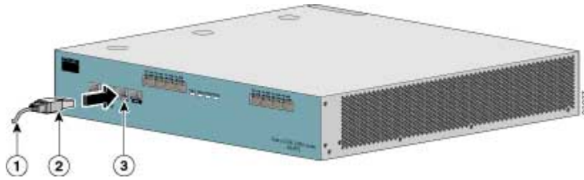
Figure 5-2: Cabling the Management Port
