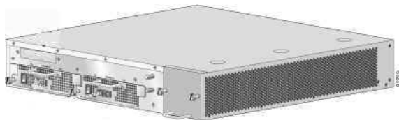
Figure 2-3: SCE Platform Back Panel: DC power
