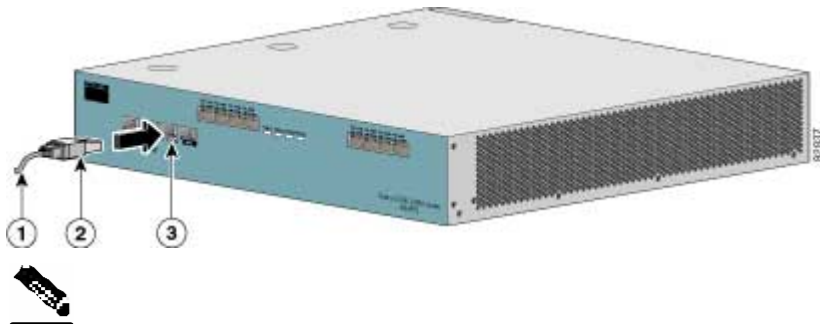
Figure 13: Cabling the Management Port
