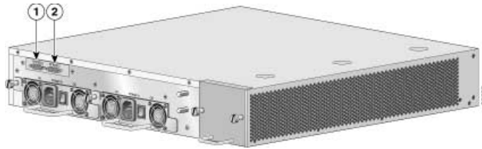
Figure A-4: Bypass Connectors on the Rear of the SCE 2000
