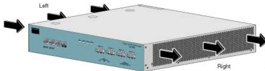
Figure 4-2: Airflow Through the SCE Platform
