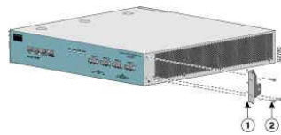
Figure 4-5: Attaching the Mounting Brackets (2-post)
