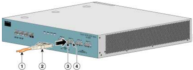
Figure 6-6: Cabling the GBE Interface
