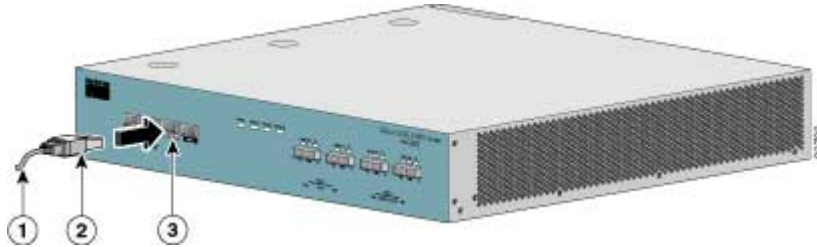
Figure 5-1: Connecting to the Local Console
