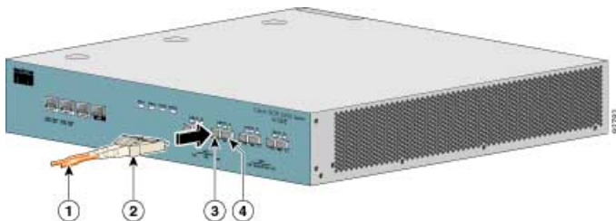
Figure 19: Cabling the GBE Interface
