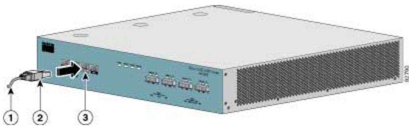
Figure 12: Connecting to the Local Console
