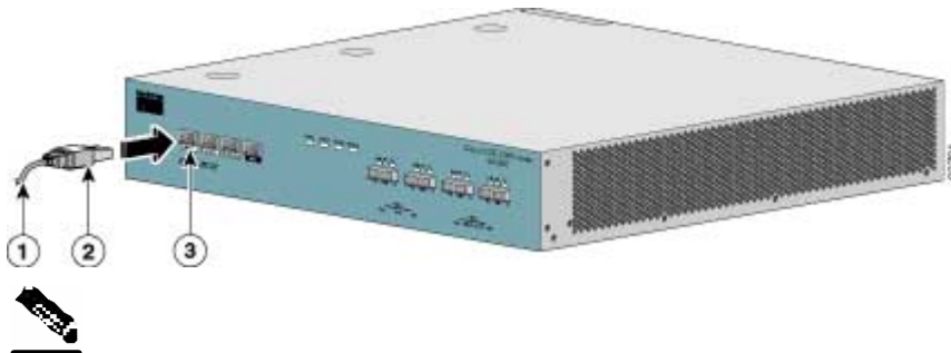
Figure 13: Cabling the Management Port
