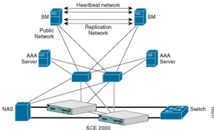
As already mentioned, an SM fail-over topology includes two SM nodes connected in a cluster scheme.
