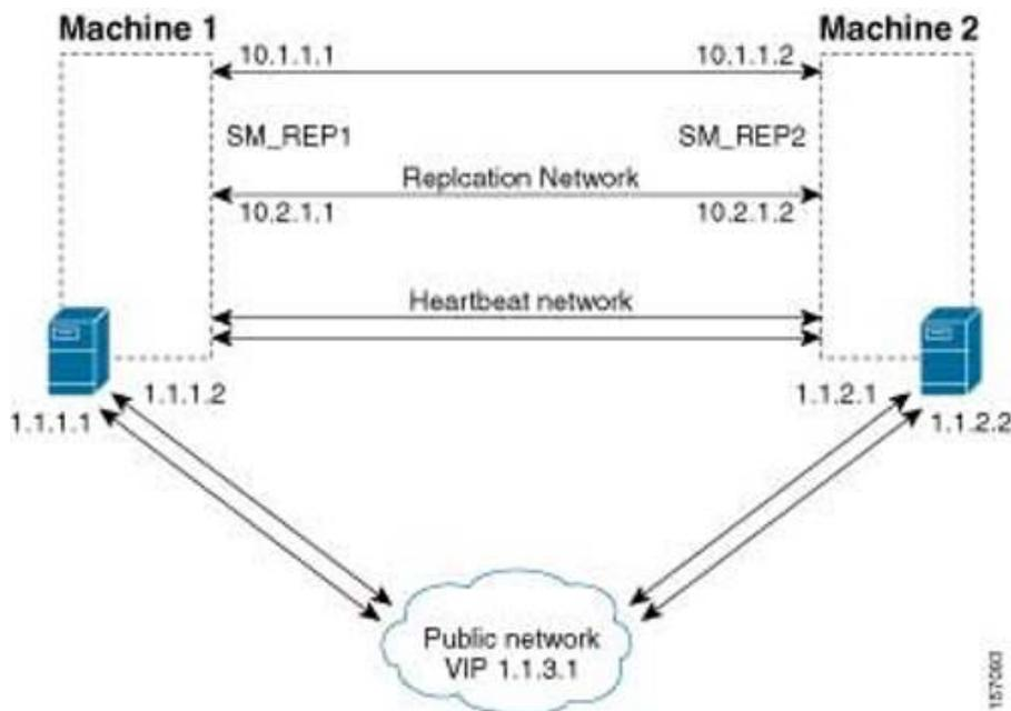
To configure the replication network shown by the above figure, do the following:
