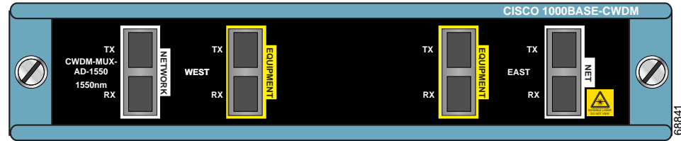
Figure 7 Dual Single-Channel OADM Front Panel (1550 nm)
