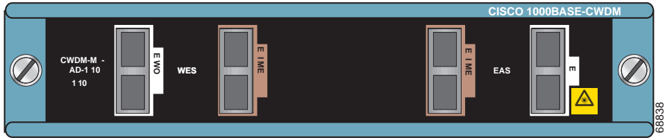
Figure 10 Dual Single-Channel OADM Front Panel (1610 nm)
