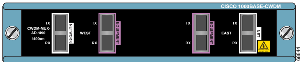
Figure 4 Dual Single-Channel OADM Front Panel (1490 nm)
