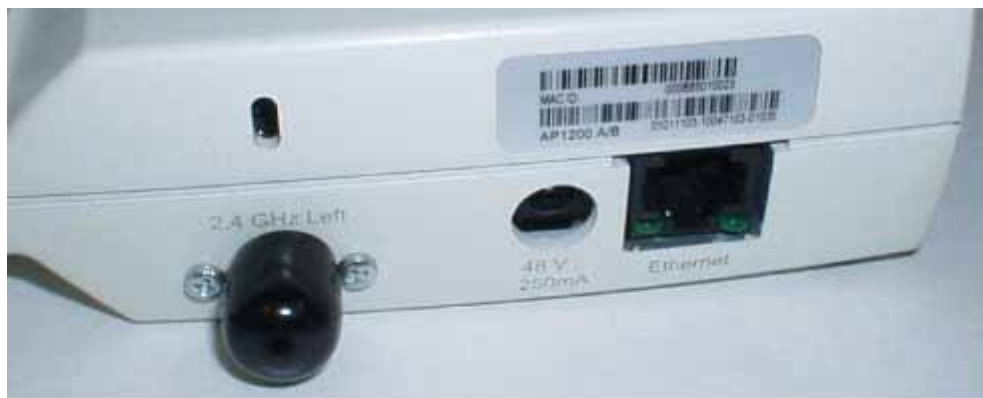
A. 2.4 GHz/802.11b Left External Antenna Port
