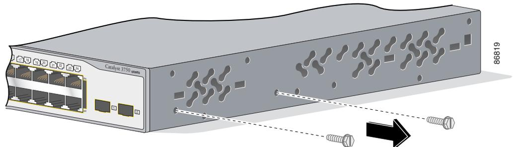
**Figure 2-10** Removing Screws from the Catalyst ,3750G-24TS-1U, 3750G-24PS, 3750G-48PS, and 3750G-48TS Switches
