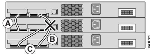
**Figure 2-4** Example of a Partitioned Stack with a Failover Condition
