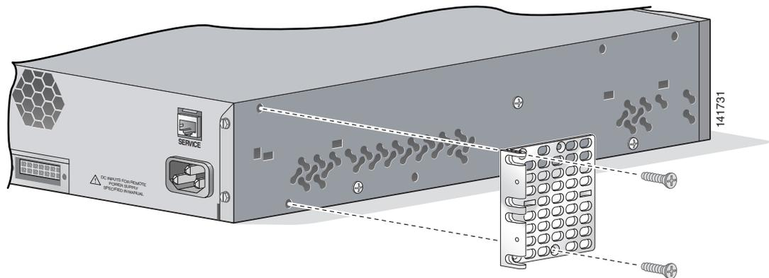
**Figure 2-22 Attaching Brackets for 19-Inch Telco Racks**
