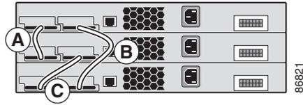
Figure 2-2 shows an example of a stack of Catalyst 3750 switches with incomplete StackWise cabling connections. This stack provides only half bandwidth and does not have redundant connections.
