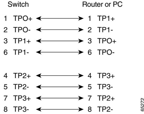
**Figure B-12** Four Twisted-Pair Crossover Cable Schematics for 10/100/1000 and 1000BASE-T SFP Module Ports
