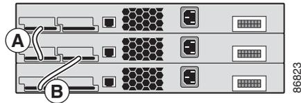
Figure 2-3 and Figure 2-4 show examples of stacks of Catalyst 3750 switches with failover conditions. In Figure 2-3, the StackWise cable is bad in link B; therefore, this stack provides only half bandwidth and does not have redundant connections. In Figure 2-4, link B is bad; therefore, this stack partitions into two stacks, and switch 1 and switch 3 are stack masters.
