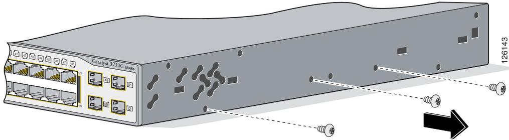
**Figure 2-11** Removing Screws from the Catalyst 3750G-12S and 3750-12S-SD Switch
