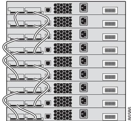
The configuration examples in Figure 2-6 use the 3-meter StackWise cable in addition to the supplied 0.5-meter StackWise cable. This configuration also provides redundant connections.
