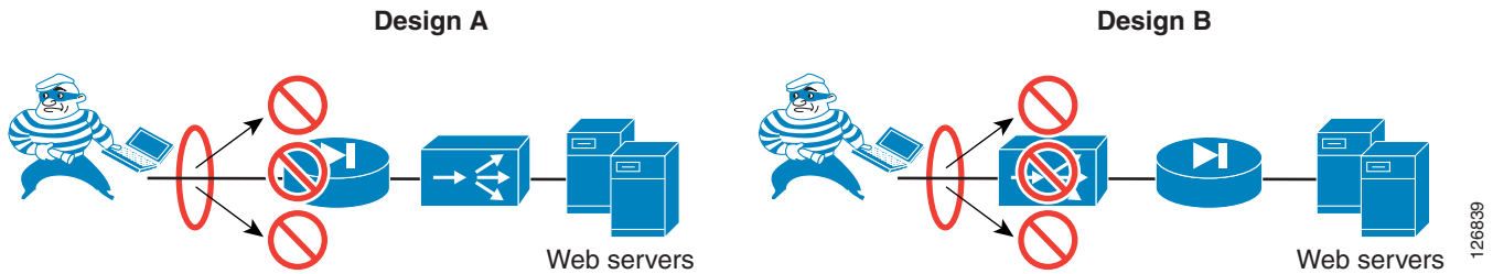
Figure 2-7 In-line Designs with Firewall and Load Balancers
