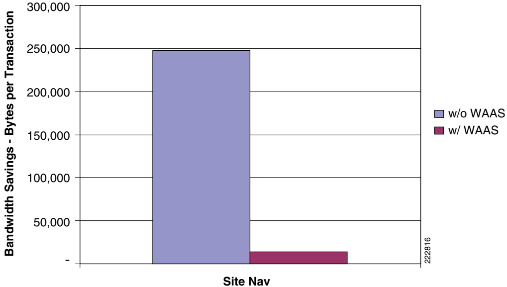
Figure 12 Bandwidth Savings for 512 Kbps WAN Link
