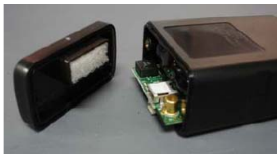
Figure 14 Assembled Tag, Battery, and Case Side View
