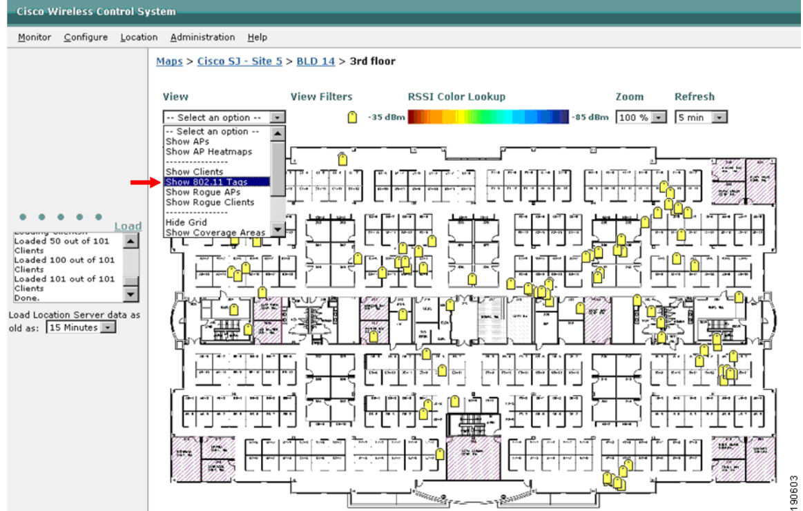
Figure 39 Enabling WCS Display of Chirp Mode Tag Location
